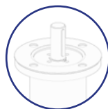
Connection F14 with shaft Ø30 mm
