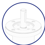
Connection F10 with shaft Ø20 mm
