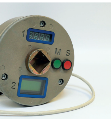
Position indicator with fibre technology and digital display.
