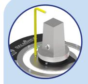
Loosen and remove the marked set screw.
